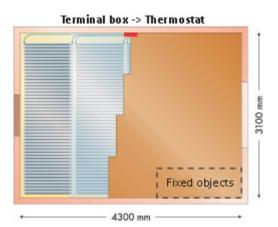
The connection leads from each strip go into the box where they are connected to the terminal board. Each set (strip of foil) has two conductors – one is black, the other one blue. Connect the blue conductors separately and the black ones separately in the
