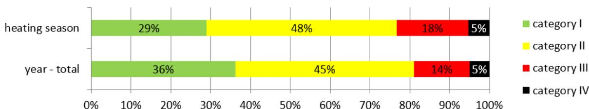
Fig.6 Footprint for relative humidity – whole building – offices
