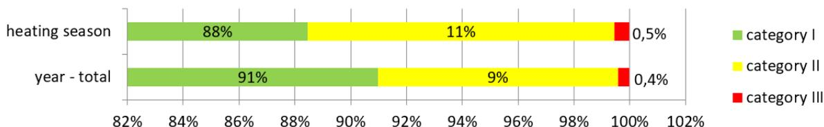
Fig.8 Footprint for CO<sub>2</sub> concentration – whole building – offices
