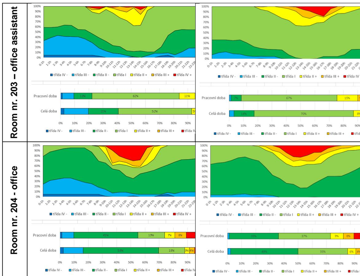
Fig.5 Evaluation and Categorization of Air Temperature in January and February 2017 in Offices
