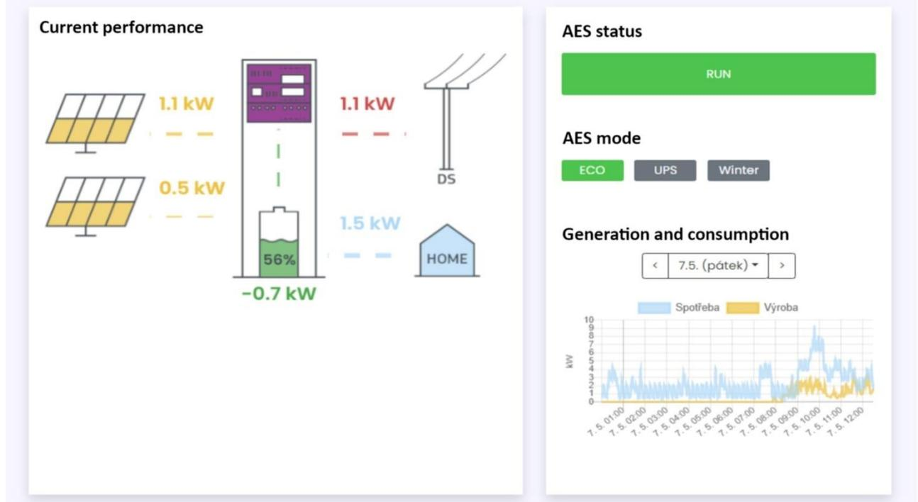
When entering the control interface, each user has an immediate view of the operational status of the station, which is shown on the “Overview” page. On this page, the instantaneous values of the operating variables in minute average are shown in individual blocks. A negative sign on the power display for batteries indicates charging at the indicated power.
