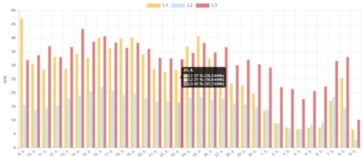
The difference of values in the individual graphs “Consumption by phases” and “Distribution consumption by phases” represents the energy delivered to each phase from its own generation.
