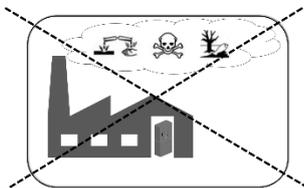
The installation site must not be contaminated with ammonia, corrosive vapours, salts or acids.
