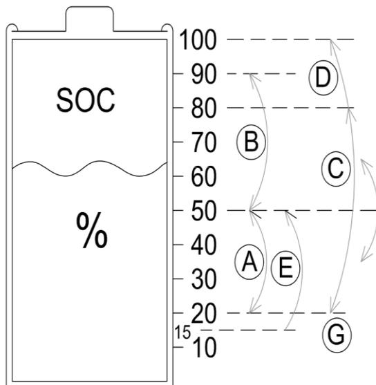
(A) – Range of 20 to 50% SOC. This range is intended for the capacity reserve of the station operation in island operation or in the operation of controlled compensation of grid consumption in times without solar energy (reduction of the power drawn from the grid, at high coincidence).
