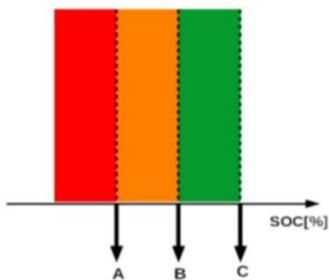
A – SOC when network charging is switched on
