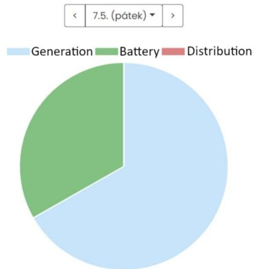
The “**Consumption coverage**” diagram shows how much the different sources, i.e. the distribution network, the solar panel generation and the energy stored in the batteries, contributed to the consumption of the building. The user has access to the exact values of the averages by placing the cursor on a specific area of the diagram.
