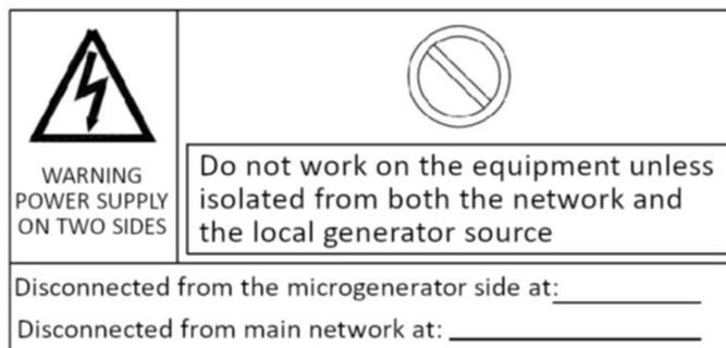
The HES6/10 station is equipped for mounting connection terminals on both the right and left side. Access to the terminal block is covered by a side plate. The position on which side the terminal block is located is marked on the respective side part with the following label according to EN 50438ed1.
