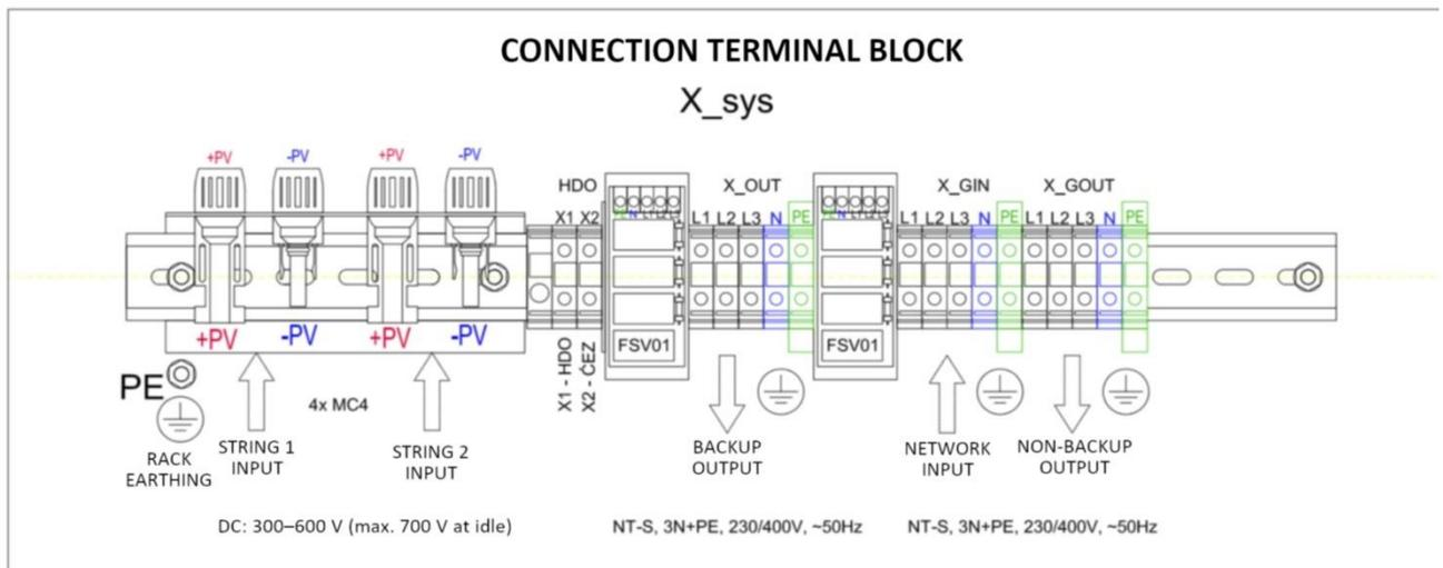
The means for disconnecting the DC leads are implemented on the X<sub>sys</sub> connection terminal block. This terminal block serves as a single point for the connection of the supply and output cable and the connection of the equipment to the internal installation of the building.
