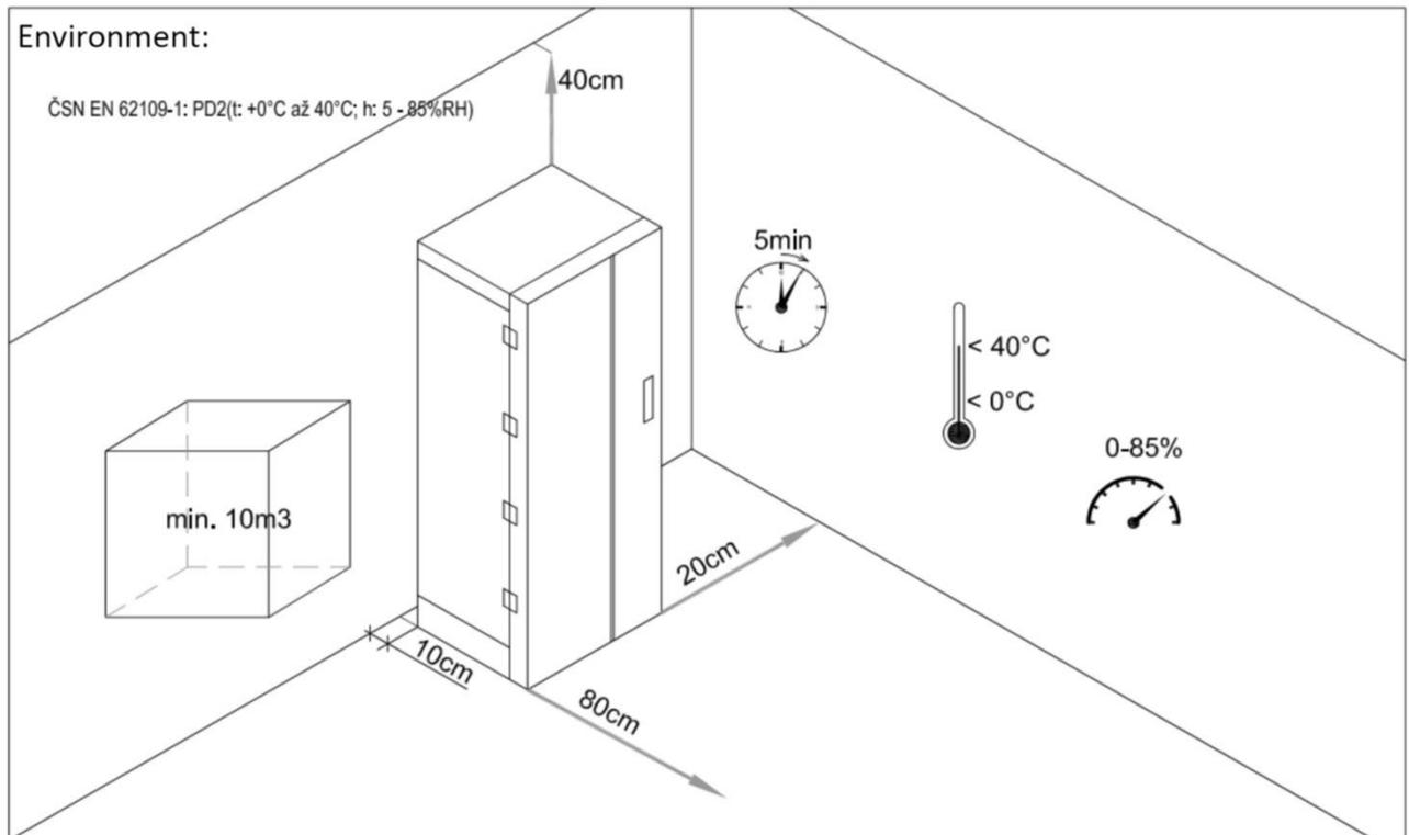
Only install the equipment on a solid surface!
