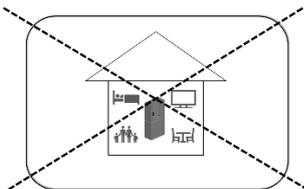
Due to the slight noise generated during operation of the equipment, we do not recommend installation in close proximity to bedrooms and living areas.
