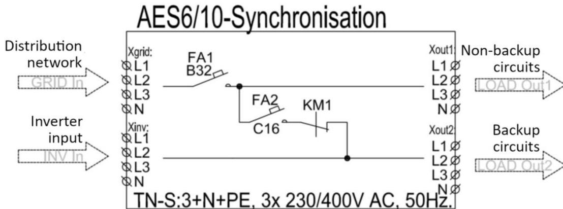
**Block diagram of the HES6/10 Synchronization unit for the purpose of documentation of the description of the HES6/10 station connection to the DN in parallel operation with the network.**
