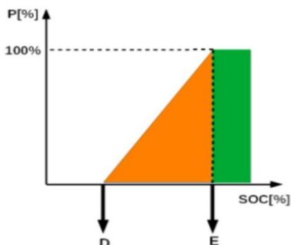
D – SOC when battery compensation starts
