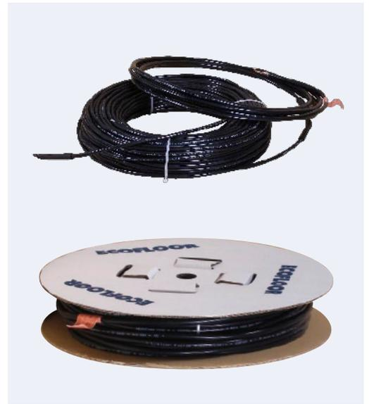
► **PSV heating cable** – a single-conductor cable with a full protection screen for storage and semi-storage heating. Cold lead 2×5 m. 230 V. Cable diameter 4.5–4.8 mm.
