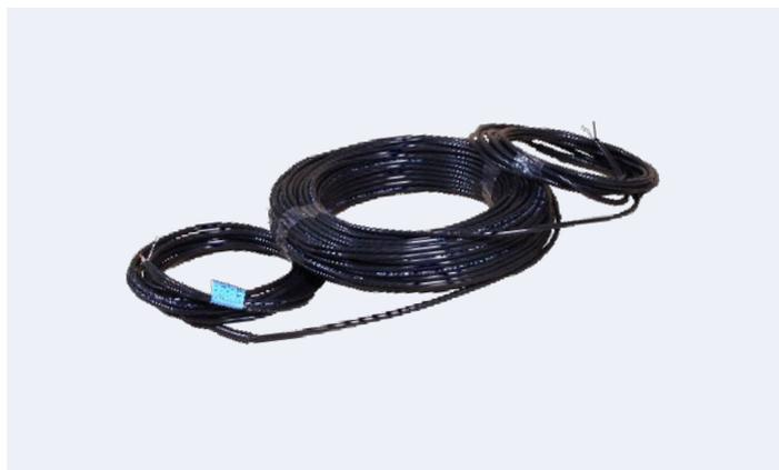
► **MADPSP heating cable / MDT heating mat** – a two-conductor cable with a full protection screen and protection against UV radiation. Suitable for heating outdoor surfaces. Class M2. Cold lead 1×5 m. Ø 6.3–9 mm. MDT heating mat: width 0.75 m. Packed in PE foil.
