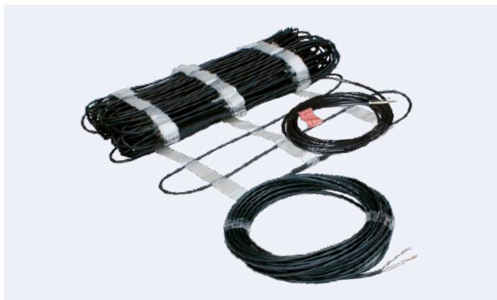
► **ADSV+ heating cable** – a two-conductor cable with a full protection screen. The sheathing of the cable is resistant against UV radiation and is intended for floor heating and the removal of snow and ice from roofs and eaves troughs. 1×3 m cold lead.  $\varnothing$  5.0 mm. 230 V.
