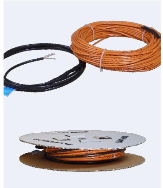
► **ADPSV heating cable** – a twin conductor cable with a full protection screen suitable for semi-storage and storage floor heating in living areas. Class M2. 1×5 m cold lead. Ø 5.3–5.9 mm. 230 V.
