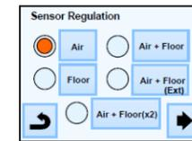
Select the chosen sensor regulation by pressing on the touch button near the sensor regulation possibilities. The active touch is colored red. Press the ▶ key in the bottom right corner to continue to the next part of the installation
