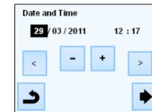
Select the time format 12H or 24H using the same method as above. Press the (◀) or (▶) keys to activate the value to be modified. Each time a value is highlighted, it can be modified by pressing the (+) or (-) keys. Press the ▶ key in the bottom right corner to continue to the next part of the installation
