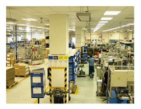
The panels are placed not only in the production halls but also in storage areas. The positive effect of radiant heating, which doesn't heat the air but the objects which the radiation encounters, can be seen here. The warming of halls with such a great ceiling height would be virtually impossible with the use of classical convection systems.
